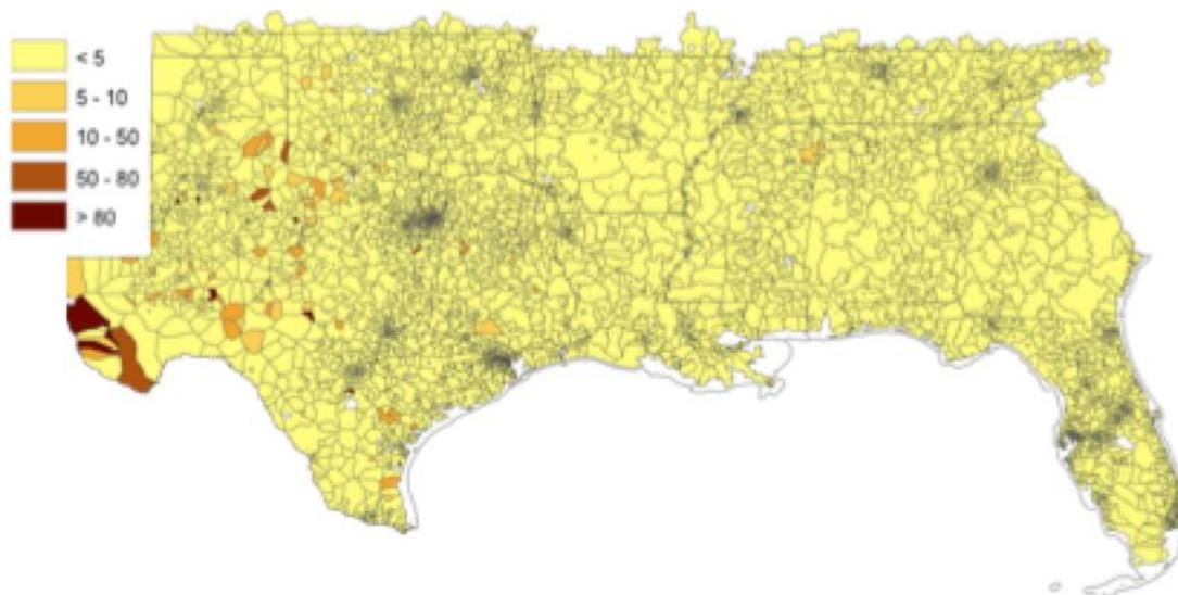
Figure 6. Per cent of substation capacity of peak electricity demand by service area in the 2050s two years after a 2005-like hurricane season.
