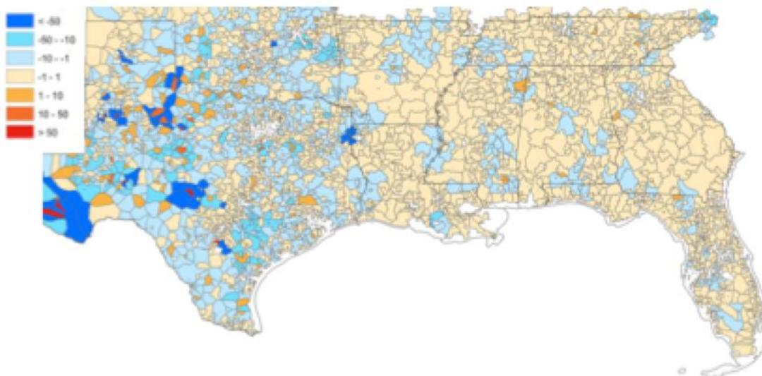
Figure 8. Difference between predicted 2050 percent capacity used during peak demand with temperature rise due to climate change two years after 2005-like hurricane event and 2011 peak demand.
