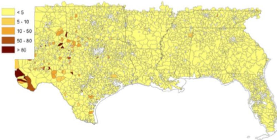
Figure 7. Per cent of substation capacity of peak electricity demand by service area in the 2050s two years after a 2005-like hurricane season and including added demand due to rise in maximum July temperature.
