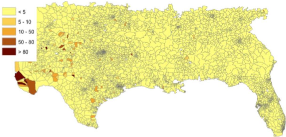
Figure 4. Per cent substation capacity used at peak demand by model-determined customer service areas in the year 2011.
