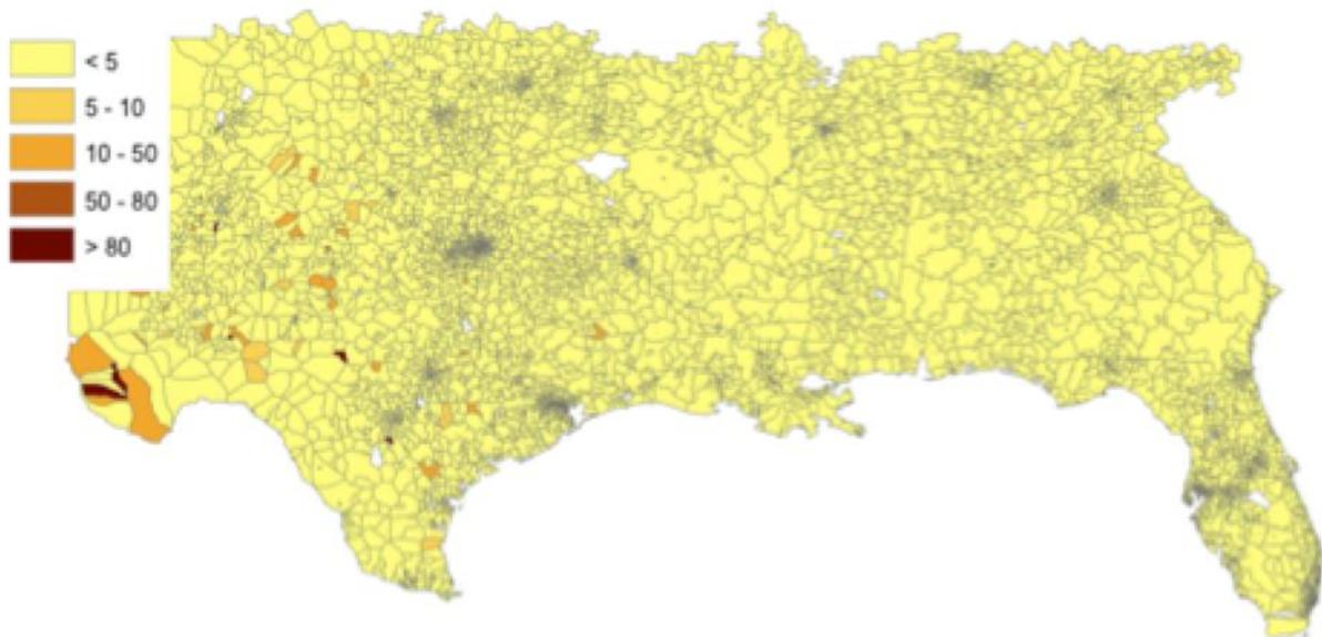
Figure 5. Per cent of substation capacity of average electricity demand by service area in 2030 if service areas are redistributed to match 2030 population distributions.
